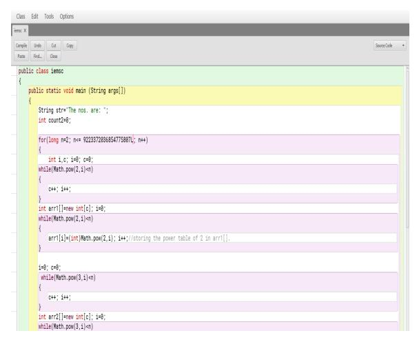
Fig1 Program code (in JAVA), for printing all the integers from 2 to 9223372036854775807, that can be be represented as  $2^x + 3^y$  in more than one way (two ways).
