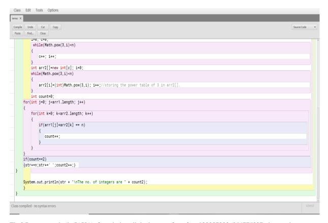
Fig.2 Program code (in JAVA), for printing all the integers from 2 to 9223372036854775807, that can be be represented as  $2^x + 3^y$  in more than one way (two ways).
