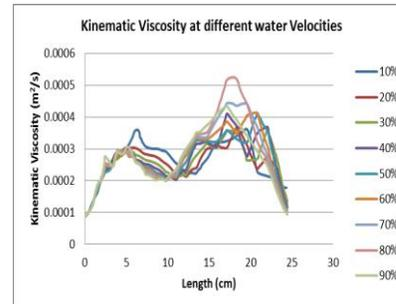
Fig 3- Kinematic Viscosity at different water velocities keeping oil velocity constant
