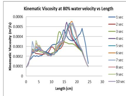
Fig 5- Kinematic Viscosity at water velocity 80% of oil velocity for 10 seconds
