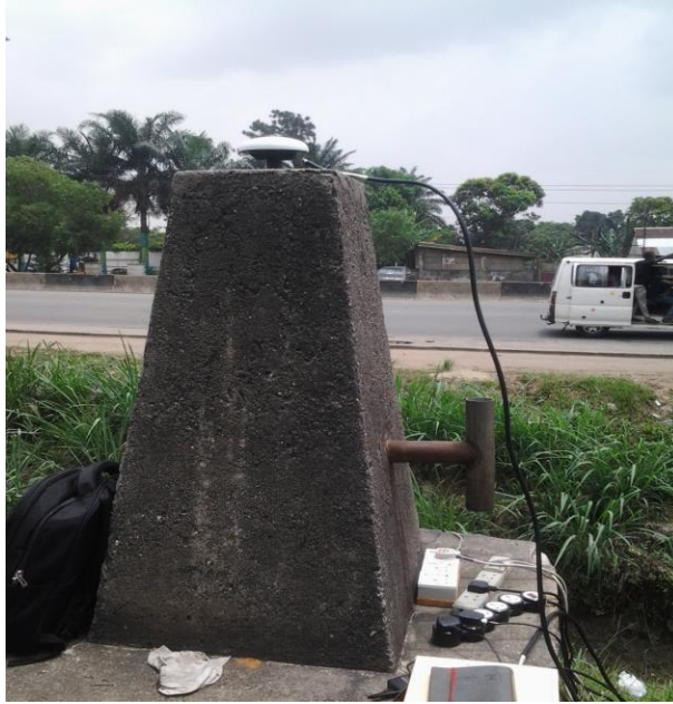
Fig 3.1: ZVS Calibration Monument (ZVS 3003 Shell Control Point, Nigeria)
