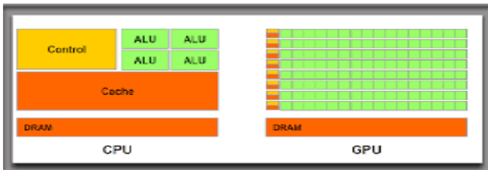
Fig 3. Pictorial Comparison of CPU and GPU Architecture
